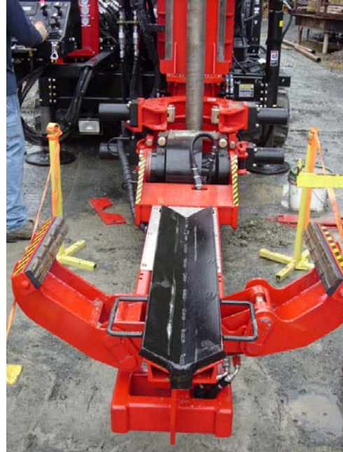
Sonic Drill Corporation's inexpensive new single rod loader eliminates heavy lifting and prevents physical contact with rotating rods.
