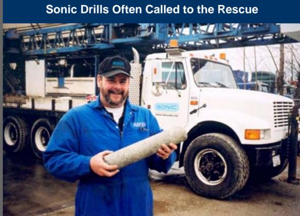
Sonic drills are often used as “rescue” drills. In one example, a sonic drill was called in replace a trio of rigs working on a geothermal project for the Langara community college in Vancouver. In the Langara case history, three standard rigs had been working the site for nearly two months and, in that time period, they had managed to drill only 18 holes in total.
