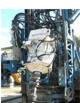
The sonic vibrations are much higher than the natural frequency of the surrounding soil and are not transmitted beyond the immediacy of the hole – unlike a pile driver hammer which can cause severe vibrations to be transmitted a considerable distance. With a sonic rig, as the outer casing is vibrated out of the hole, concrete is forced to flow into the void created by the casing.
