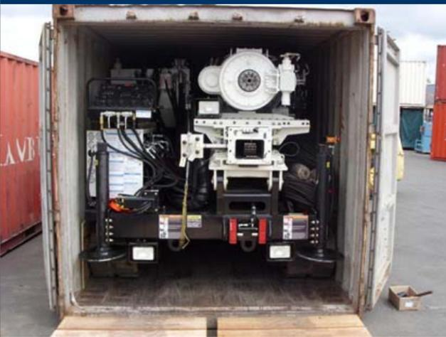
Sonic Drill Corporation, a leader in sonic drilling technology, recently released a sonic drill rig that is able to fit within a 20' shipping container.
