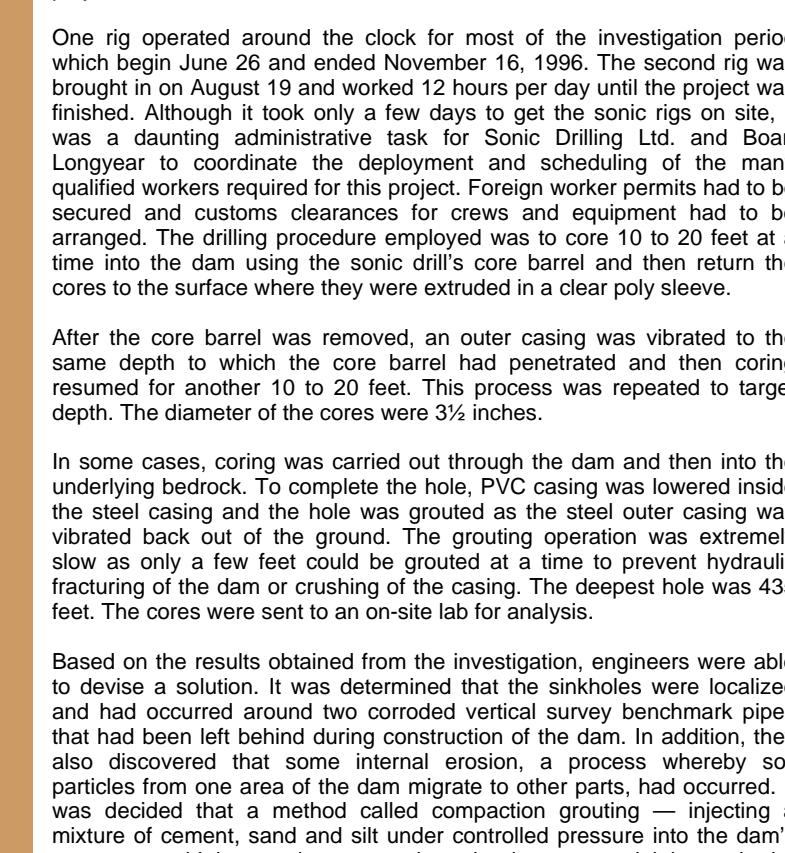
On June 14, 1996, a tourist discovered a sinkhole on the crest of the W.A.C. Bennett dam in northeastern British Columbia, Canada. This 1½-mile-long dam is a massive structure that holds back 75 billion cubic yards of water in the Williston reservoir. At 600 feet high and 2600 feet wide at the base, it was constructed as a megapower project 45 years ago and it's still one of the largest hydroelectric dams in the world, capable of generating 2,730 megawatts of electricity at peak capacity.
